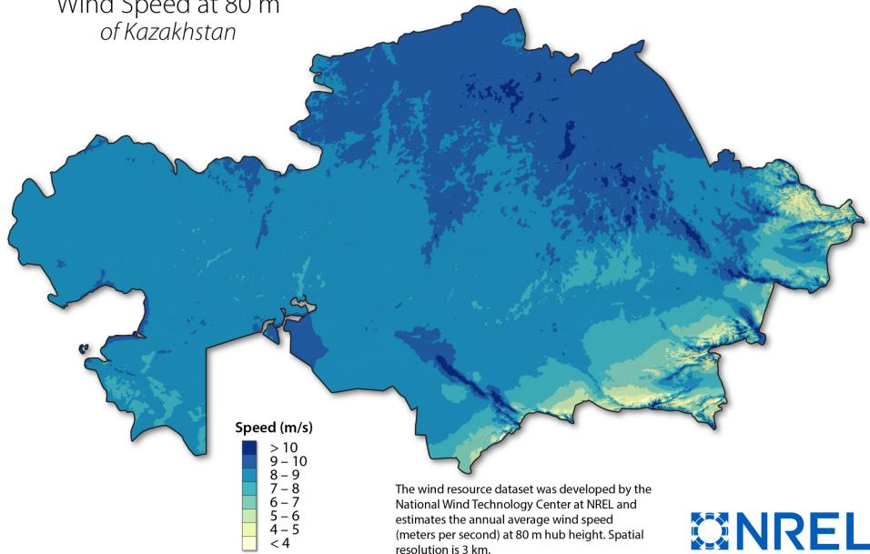
The wind resource dataset was developed by the National Wind Technology Center at NREL and estimates the annual average wind speed (meters per second) at 80 m hub height. Spatial resolution is 3 km.
